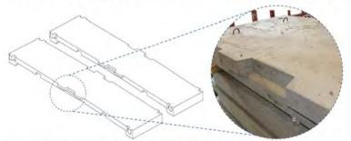
Figure 1 Shear keys in a dry deck joint in a large scale test specimen.
