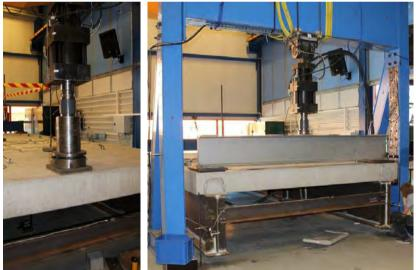
Figure A.14 The two different ways of applying the load on the specimen.
