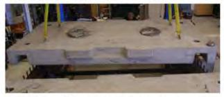
Figure 2 Picture of a dry deck joint in a large scale test specimen.
