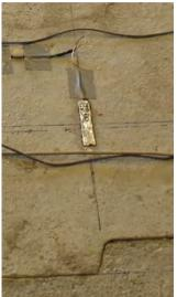
**Figure A.28** Strain gauge on top of the concrete.
